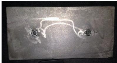
Embedded Nuts on the Back side of the Wear liner Eliminates the surface hole where wear begins.
