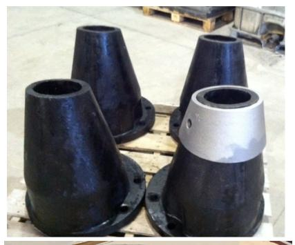
Mud Gun Nozzles and Collars are available in ductile iron and standard Gray iron
