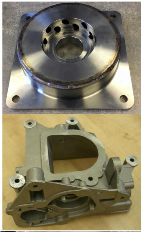
Stainless Steel Burner Nozzles for reheat Furnace. 96 sets produced from reverse engineered original
